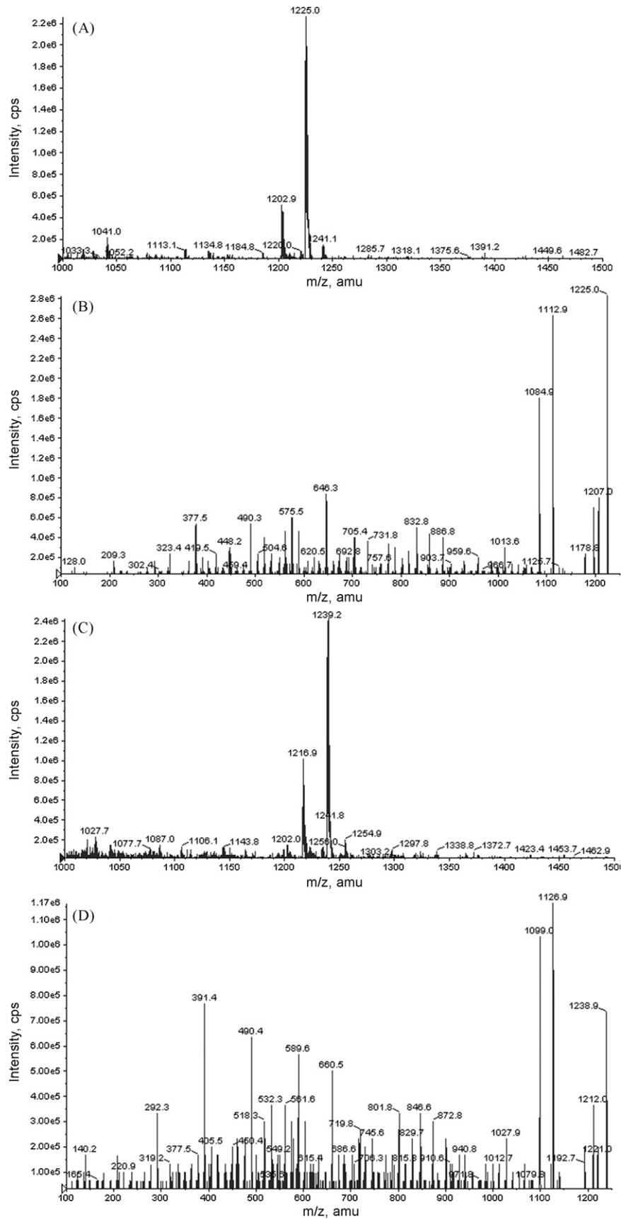
**Fig. 1.** Mass spectra of CyA and CyD. (A) Enhanced mass spectrum of CyA; (B) enhanced product ion spectrum of  $[M+Na]^+$  of CyA at m/z 1225.0; (C) enhanced mass spectrum of CyD; and (D) enhanced product ion spectrum of  $[M+Na]^+$  of CyD at m/z 1239.2.
